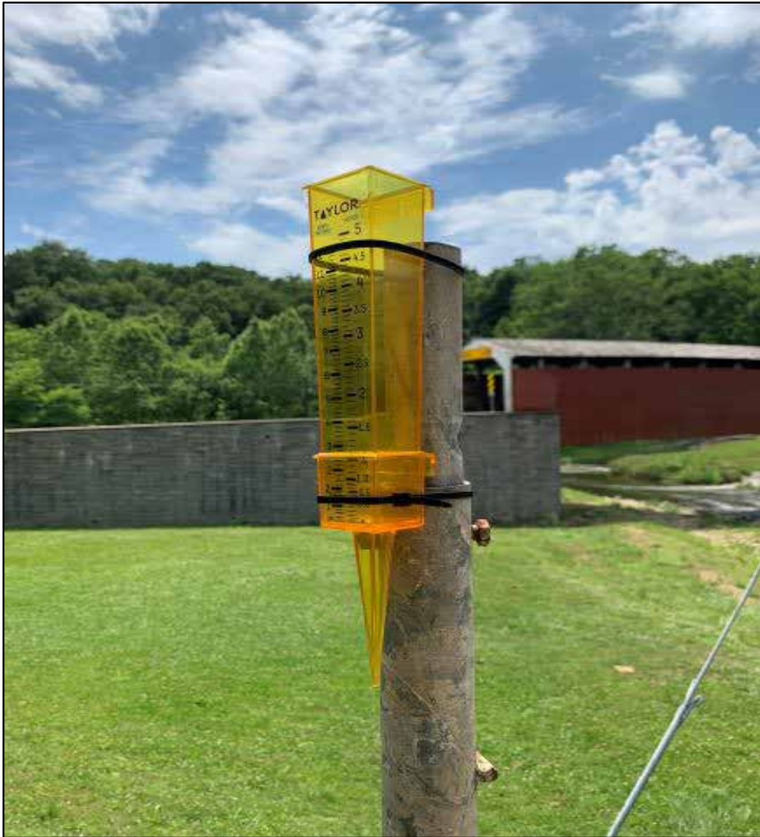
Figure 3.1-2: Rainfall gauge, Octoraro Creek Eel Facility, 2021
