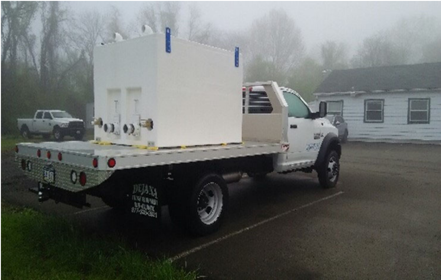
Figure 3.6-4: Large Eel Transport Tank, Conowingo West Eel Collection Facility, 2021
