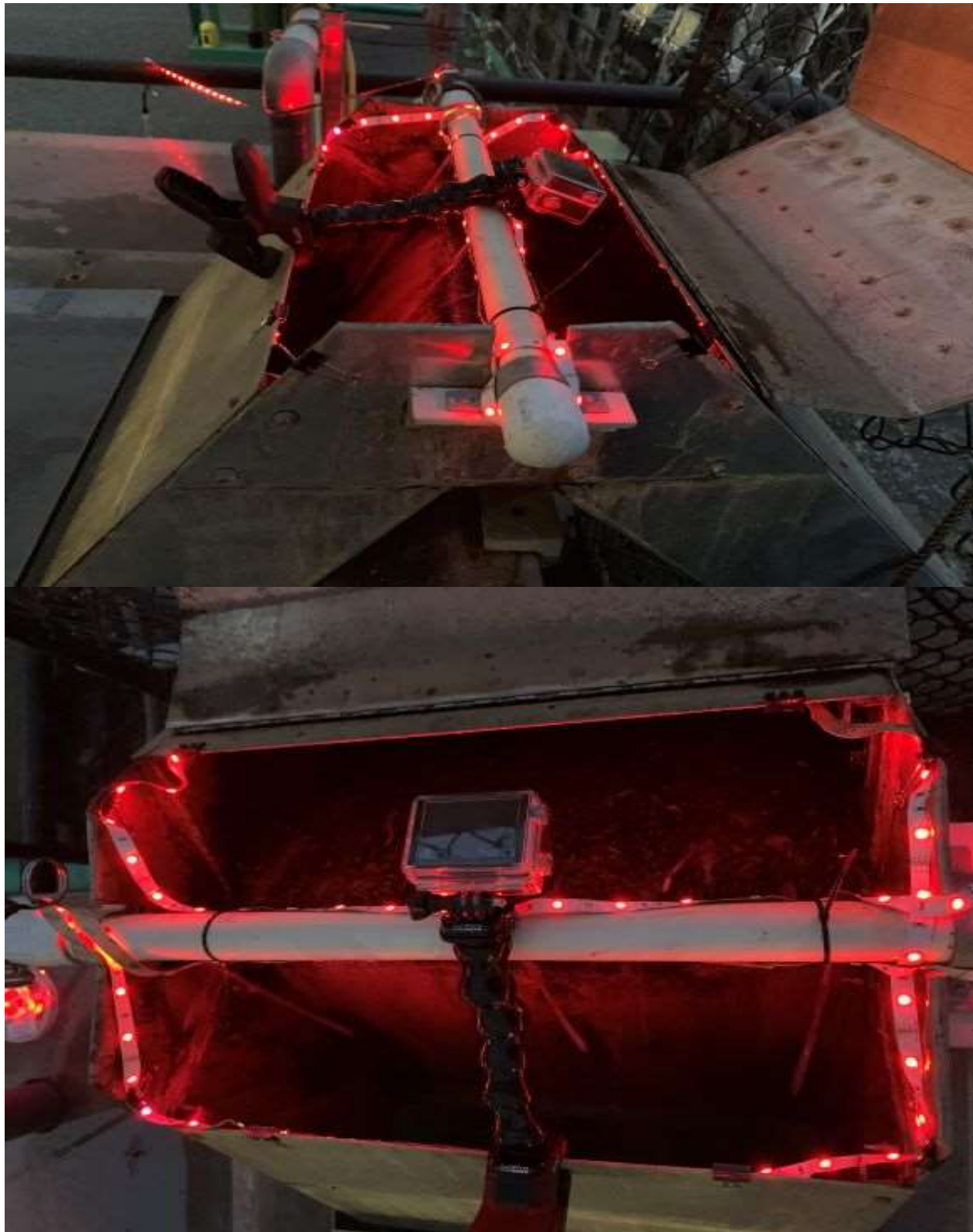
Figure 1: Position of the Go Pro Video Camera and the Minger RGB LED Strip Lights at the Top of the Ramp, Conowingo Eel Collection Facility, July 2020.
