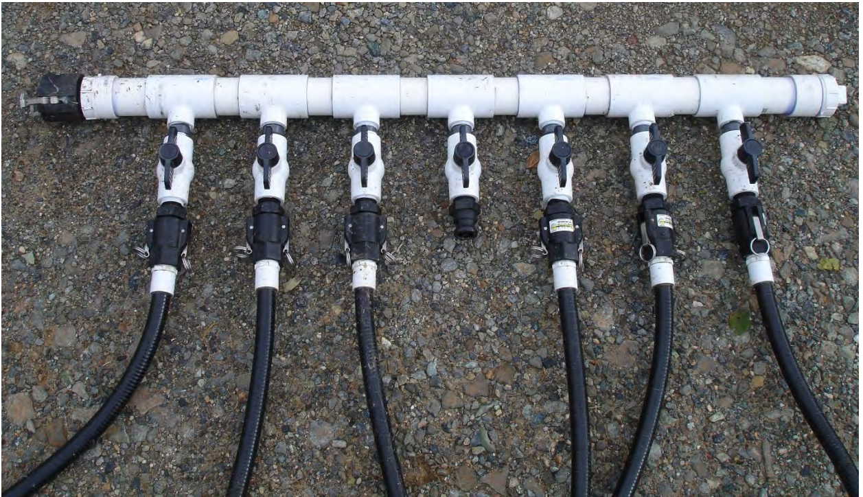
Figure 3.1-4: Upgraded Manifold and Attraction Line, Octoraro Creek Eel Facility, 2019
