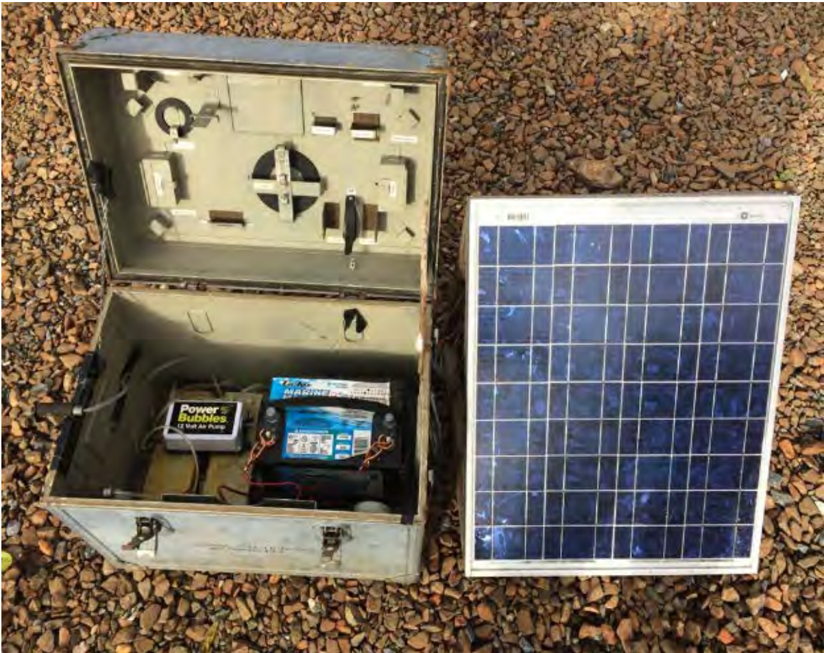
Figure 3.1-6: Aerator Powered by a Marine Battery and Charged by a solar Panel, Octoraro Creek Eel Facility, 2019
