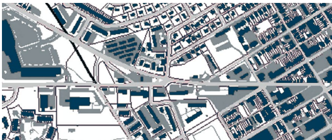
Mapping impervious surfaces with lidar data. Surfaces were classified as Buildings, Roads, and Other Impervious Surfaces.
