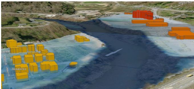
FEMA 100-year floodplain near Johnstown, PA displayed with 3D buildings. Building colors show the dollar loss estimate, with higher values in orange and red. Source: Cambria County GIS Center.
