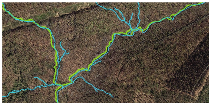
Comparison of the current stream mapping (green) to lidar-derived streams (blue). of the Upper Chiques Creek, Lancaster County.
