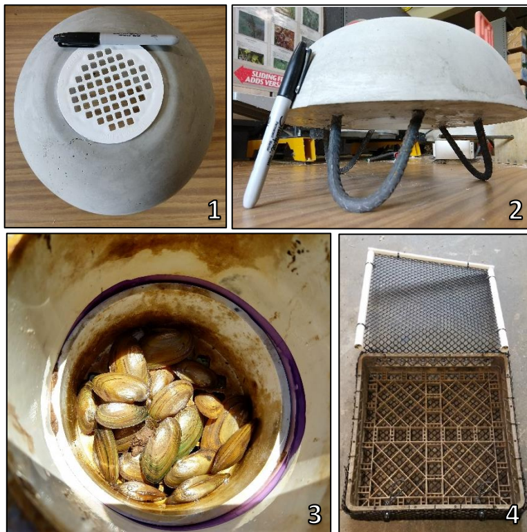
Figure 4.1: Examples of in stream Silo (1-3) and Benthic (4) mussel cages from Partnership for Delaware Estuary (PDE)
