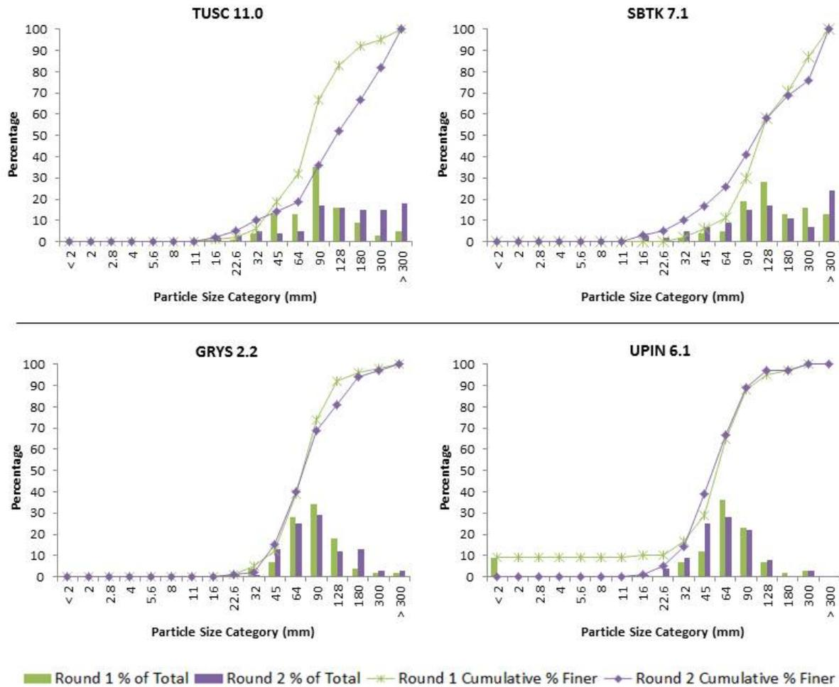
Figure 7. Substrate Particle Size Distribution (Percentage of Total and Cumulative Percentage Finer) for TUSC 11.0, SBTK 7.1, GRYS 2.2, and UPIN 6.1, Comparing Round 1 and Round 2 Pebble Count Data
