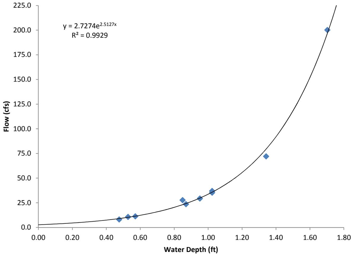
**Figure 3. Preliminary Flow Rating Curve for the DRFT 2.0 (Driftwood Branch Sinnemahoning Creek) Flow Monitoring Network Station**
