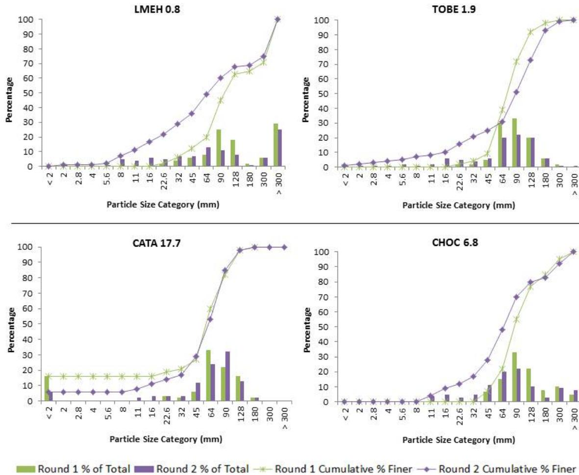
Figure 6. Substrate Particle Size Distribution (Percentage of Total and Cumulative Percentage Finer) for LMEH 0.8, TOBE 1.9, CATA 17.7, and CHOC 6.8, Comparing Round 1 and Round 2 Pebble Count Data
