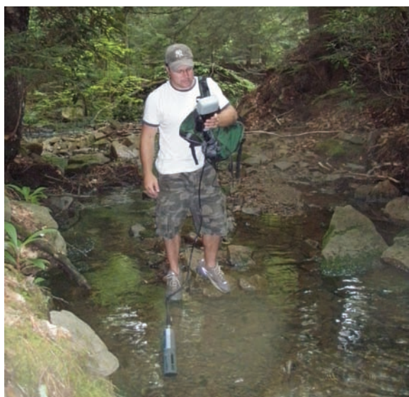
Field chemistry parameters (temperature, pH, conductivity, and dissolved oxygen) were measured instream using a YSI 6820 multi-parameter meter.
