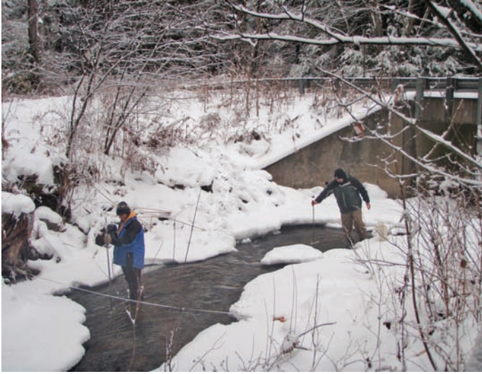
SRBC staff collects a water sample and takes a flow measurement in Drury Run during January 2010.
