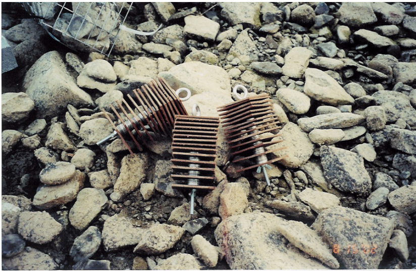
Figure 4. Multi-plate Samplers Used in River Assessment Project
