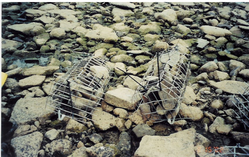
Figure 3. Rock Baskets Used in River Assessment Project
