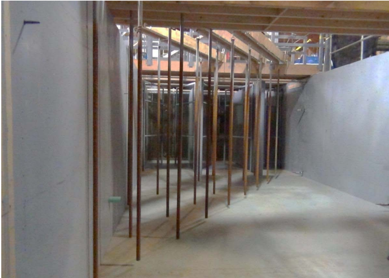
Figure 4-1 Downstream view of three electrode arrays used for evaluation of eel responses to behavioral cues. In the first (upstream) array of electrodes, the ninth electrode (at far right) was added for Block 4 and 5 trials. The FVES eductor nozzle can be seen on lower part of the left hand wall near the first electrode in the second array. One set of surface and bottom hydrophones can be seen on right hand wall just upstream of the bypass collection bin entrance and surface hydrophone can be seen protruding from the temporary (left) wall in the upper left corner of the photo.
